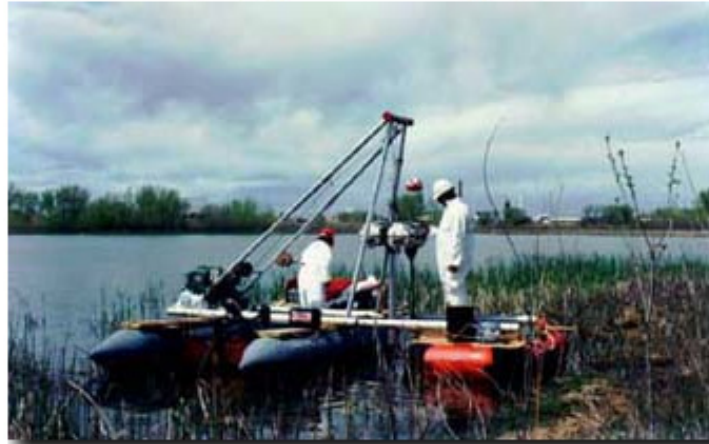
Vibrocoring on Small Inflatables in Marsh
