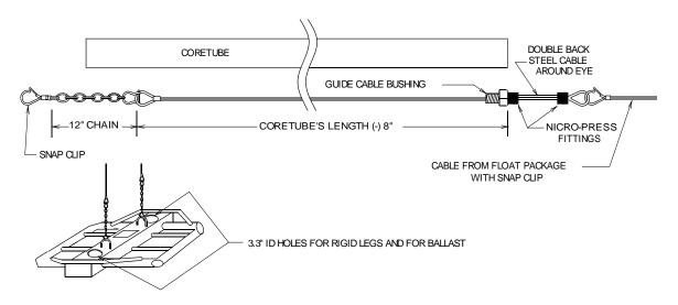
5. When the guide cables are properly adjusted, the corenose on the end of the coretube when mounted in the vibrohead should be captive inside the guide tube of the weightstand by approximately 2-3" from the top. The corenose does not protrude under the weightstand.
