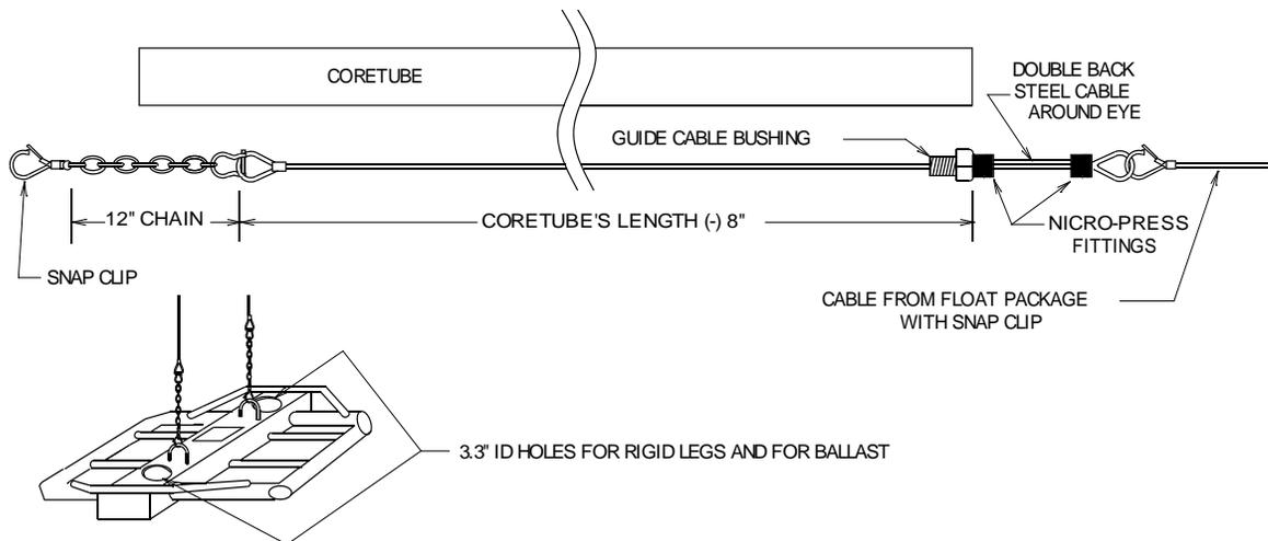
5. When the guide cables are properly adjusted, the corenose on the end of the coretube when mounted in the vibrohead should be captive inside the guide tube of the weightstand by approximately 2-3" from the top. The corenose does not protrude under the weightstand.
