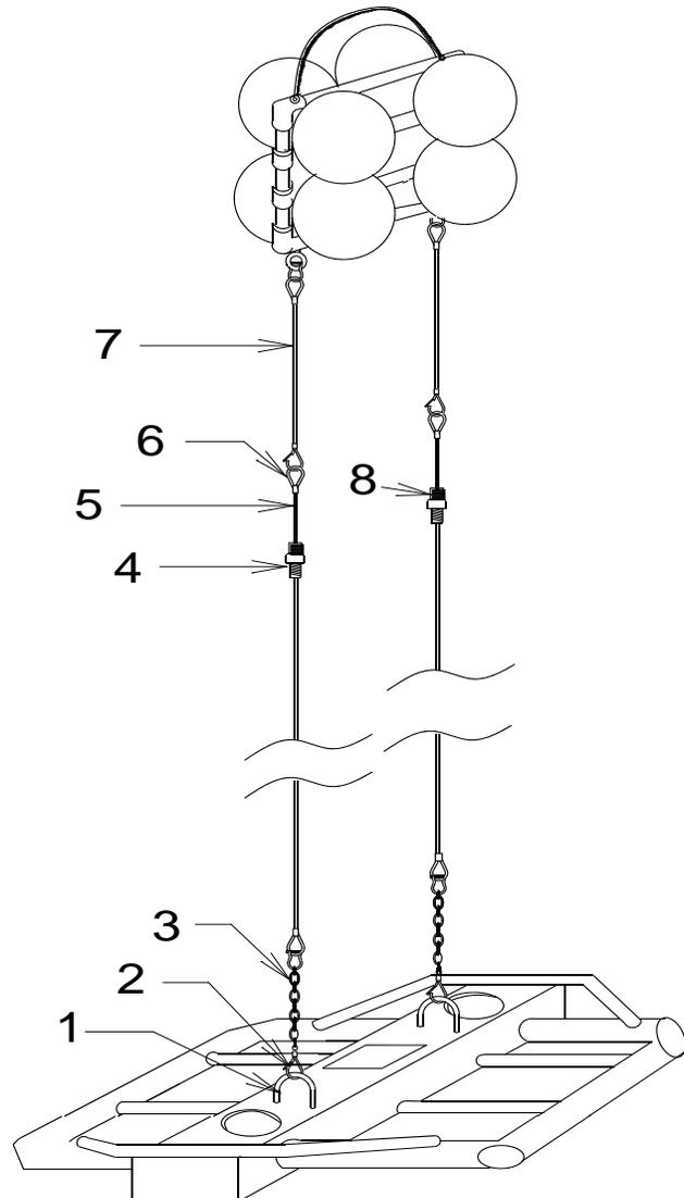
For deployment at sea, the most practical procedure is to deploy the Vibrocorer clipped with the guide-cables and weightstand, but without the float package. Lower this unit until the Vibrohead is level with a person's chest
